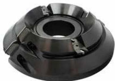
**Application:** Mitre jointing cutterhead for softwood and hardwood in longitudinal and cross direction of the fiber, coated, veneered and uncoated wood base materials such as chipboard, plywood and MDF. For corner joints with wood from 14 to 34 mm thickness in wooden boxes, drawers, etc.
