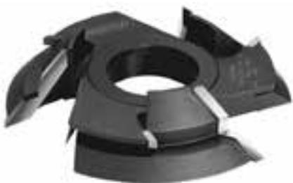
**Application:** Mitre jointing cutterblock for softwood and hardwood in longitudinal and cross direction of the fiber, coated, veneered and uncoated wood base materials such as chipboard, plywood and MDF. For corner joints with wood from 14 to 32 mm thickness in wooden boxes, drawers, etc.
